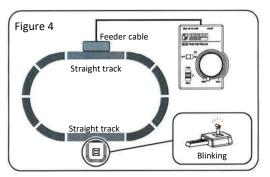
\* If the controller is RC-004, the LED will be dimmer than when using RC-02 or RC-03.
