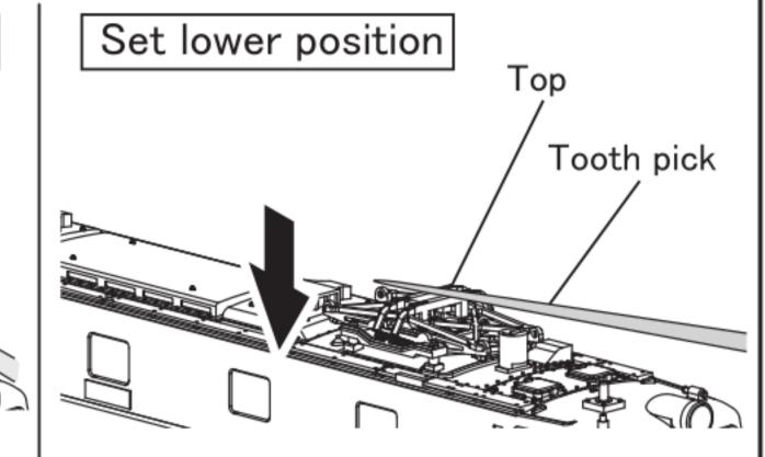
Lift-up top part softly by tooth pick until stop. Pantograph will be broken if lifting-up too much.
