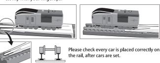
\*Use the rerailer when you put cars on the rails. By sliding wheels to groove of the rerailer, it helps easier to put on the rails. Please put in order of Head cars, Middle cars and Tail cars.
