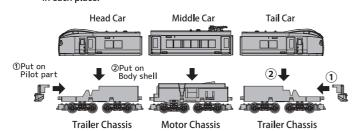
\*Some cars do not have pilot parts (1). Take Arnold couplers off trailer chassis and motor chassis, and put drawbars in.
