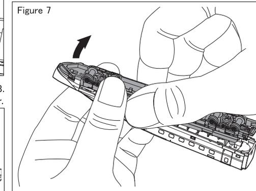
3. Set the Room Light on Chassis Unit according to Figure 8. Then, reassemble body on Chassis Unit again with reverse order.
