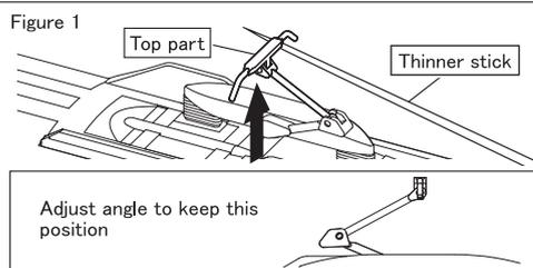
\* Pantograph will be broken if pull-up too much.
