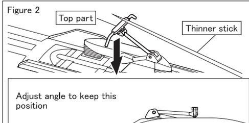
\* Pantograph will be broken if push down too much.
