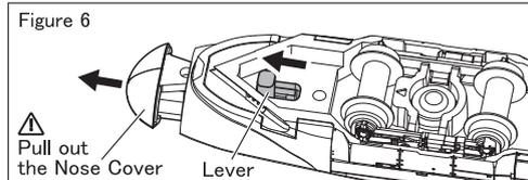
2. Pull up slightly the rear side of body from Chassis Unit first, then pull up the front side of body like figure.
