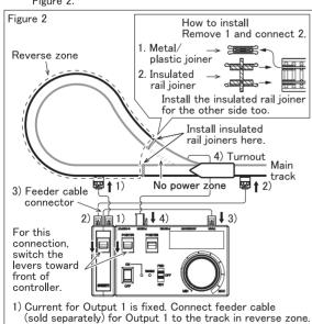
2) Current for Output 2 is switching type. Connect feeder
