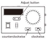
Push right hand button, then the table will turn clockwise. Push left hand button, then the table will turn counterclockwise. When push each button one time, it turns by 15 degree. When push both buttons at a time, it turns clockwise by 180 degree.
