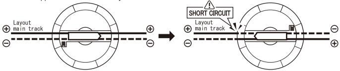
To avoid short circuit, gap joiner is necessary.
